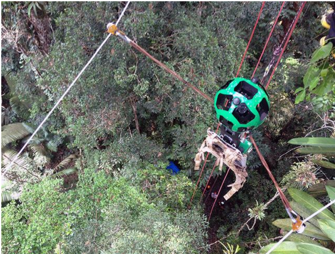
This is a zip line used to transport a camera through the Amazon Rainforest for scientific observation.
